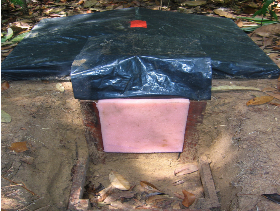
Image 1) Installed rhizotron showing foam and black plastic sheet used to minimise temperature variation and light/water entry at the perspex face. The entire rhizotron is shielded by a larger black plastic cover.
